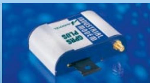
Transmission and reception of data - fax - sms - voice - internet access from every industrial device equipped with a V.24 RS232 serial port
